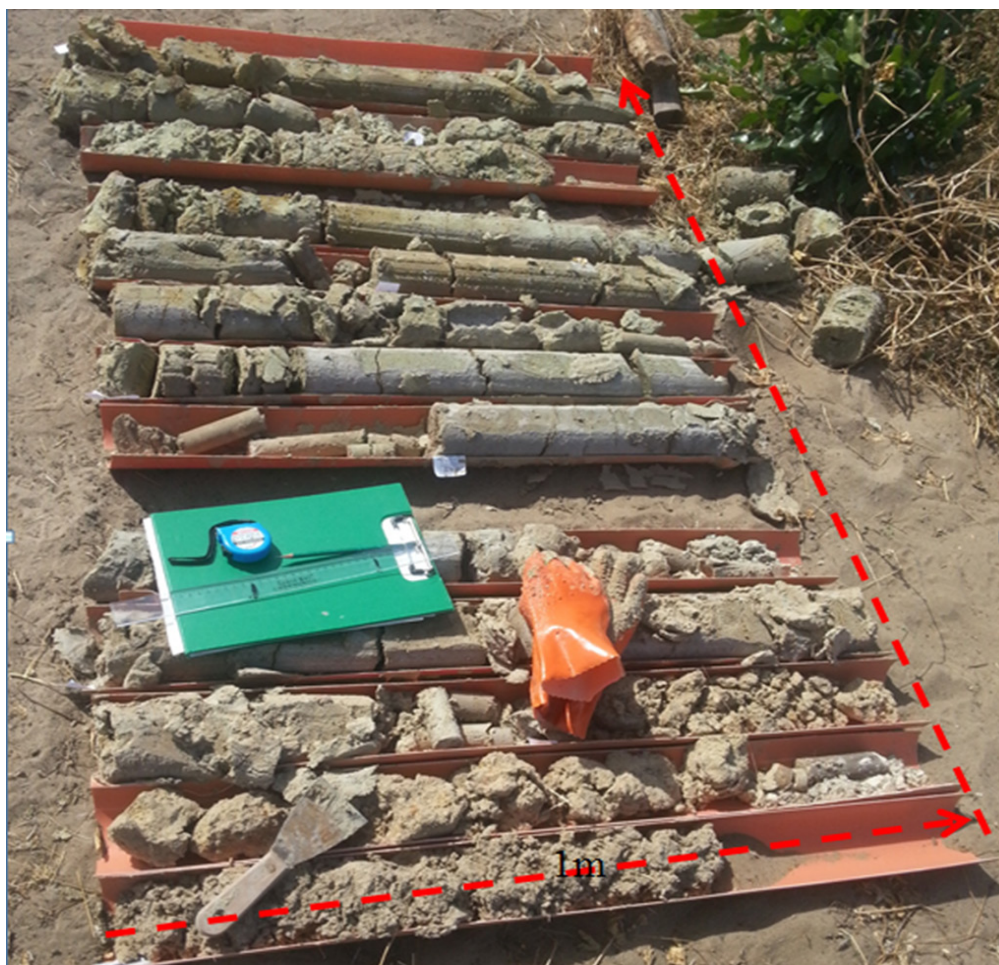
Figure 4-4: Log samples from core drilling site 2 showing fine sands (By Chinese Geotechnical Team, 2015).
