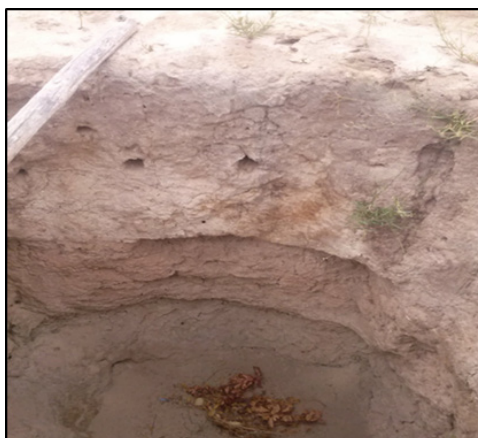
Figure 4-1: Dry well 2m deep brown-grey fine sandy soils and weathered coral limestone
