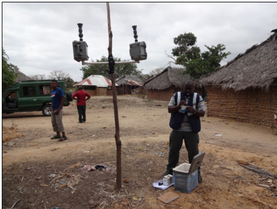
Figure 5-5: Image of Minivol air sampler mounted to collect particulate matter
