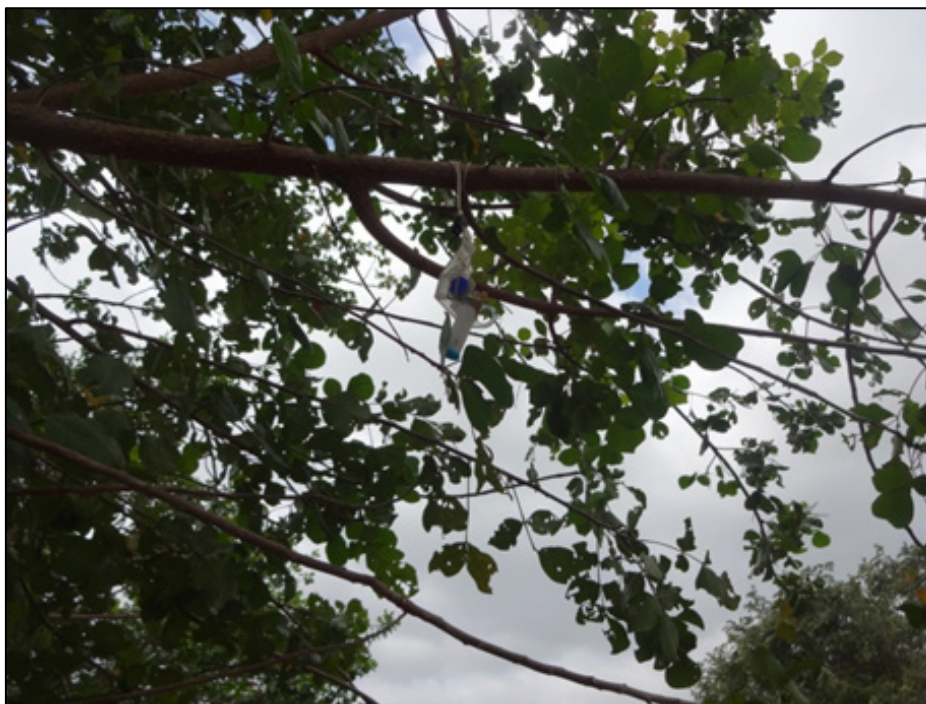
Figure 5-4: Image showing passive diffusion tubes mounted on a tree branch
